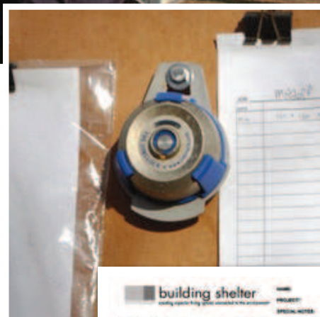
Figure 1. To record his hours, a worker simply touches the time clock (left) with an electronic fob. Handwritten time sheets (lower left) are a thing of the past.
